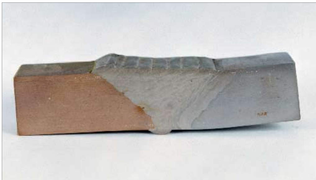
Figure 3 . Macro of a PQR sample of an 'exotic' joint in a desalination installation. 22 mm thick Cu/Ni 90/10 (left) connected to 20 mm thick S 31803 duplex stainless steel (right), welded with manual TIG with automatic wire feeding. The duplex side is first buffered with two layers of OK Autrod 19.92 (ERNi-1) followed by two layers of OK Autrod 19.93 (ERNiCu-7). Subsequently, the two sides are joined with OK Autrod 19.49 (ERCuNi). One layer, with the (acceptable) pore, is welded with MIG, just to get the process approved.
