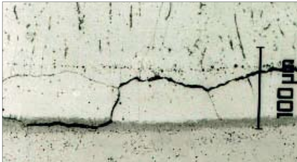
Figure 2. Disbonding in the interface region between parent material (bottom) and an austenitic overlay weld metal (top) [1].
