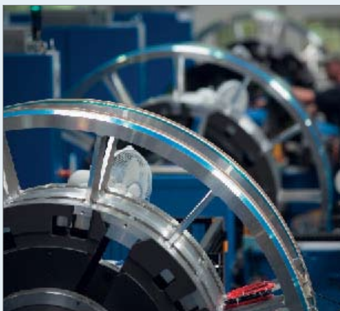
Figure 2. Superconducting magnet coil to be contained in the helium vessel.
