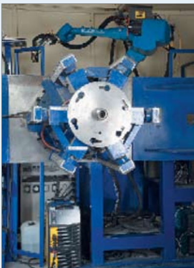
Figure 3. Motoman robot equipped with the Aristo™ robot package and internal clamp/manipulator.
